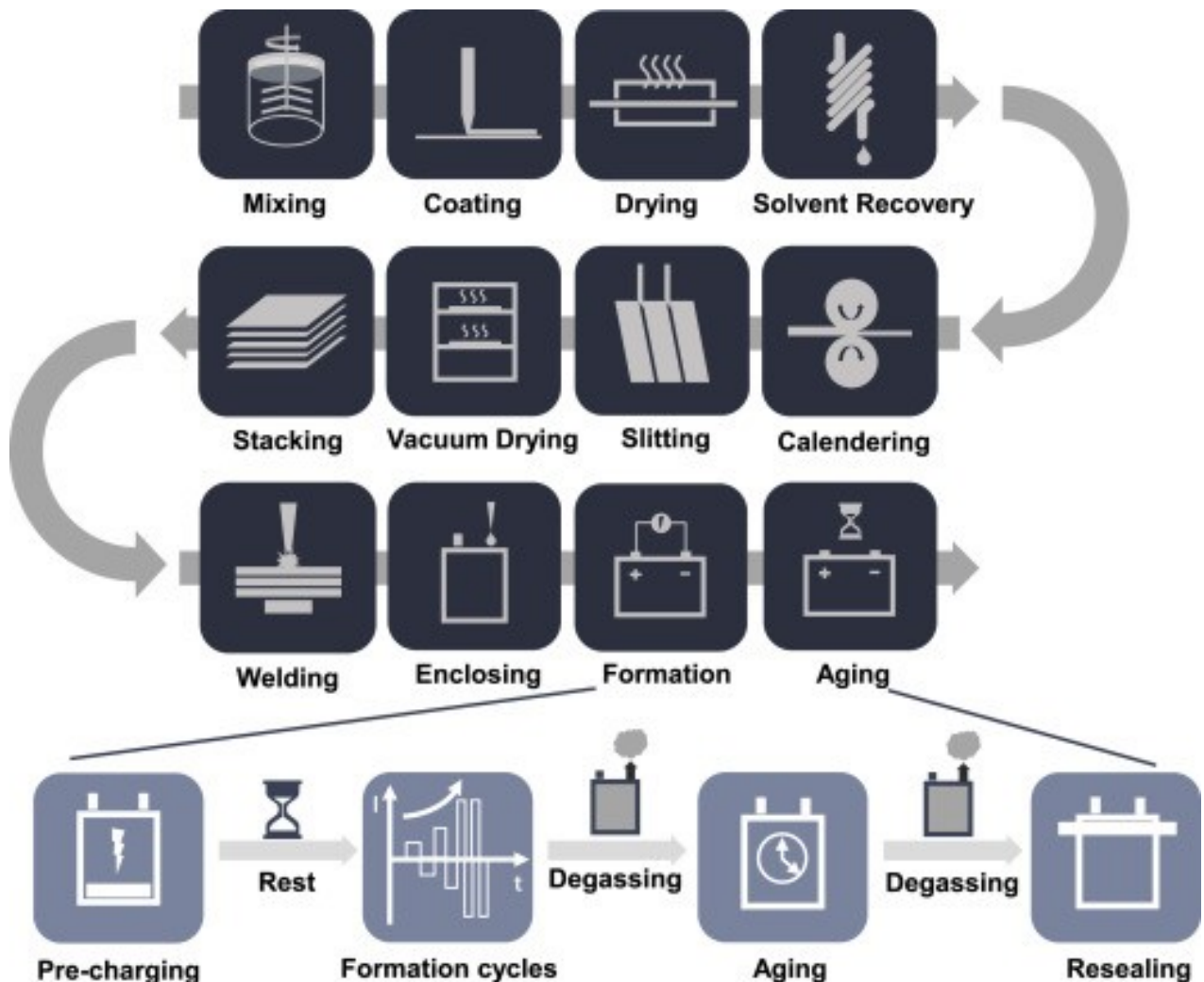
Exhibit 107: Battery manufacturing process for pouch production
